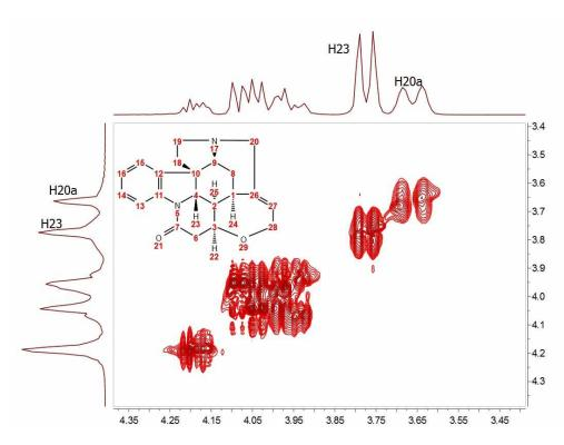
In this case, we have extended the t1-FID from 128 to 512 data points and then zero-filled up to 1024. Now we can see that the f1-lines are narrower but the couplings cannot be resolved yet.
