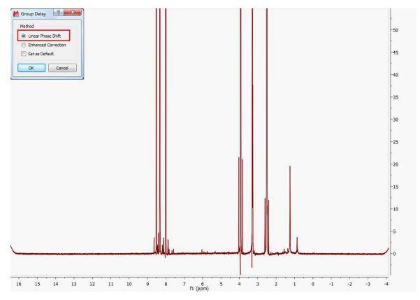
From version 6.1.0 onwards, Mnova includes a new correction algorithm (Enhanced Correction) which produces a normal and physically correct FID in such a way that the smiles/brownies will not be seen in the f-domain spectrum.
