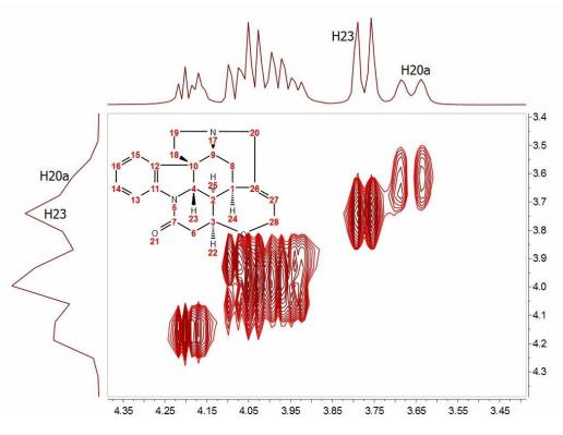
**How could this be improved?** We could try to extrapolate the FID (somehow) along the columns (F1) to a higher number of points (e.g. 1024). A well known technique is simply to add zeros, a process
