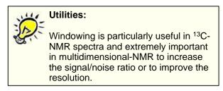
The Window function is applied by multiplying the data vector d, element by element, by a vector a. Thus element k of vector d is multiplied by element k of vector a to yield element k of vector d'.
