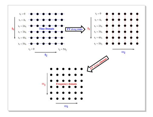
As you can see in the picture above, the first step is the application of the FT along the rows of the matrix; to obtain a new matrix (*interferogram*) where each row corresponds to an increasing value of  $t_1$  and each column to a running frequency variable  $\omega_2$ . Next the columns are subjected to a FT to obtain the final matrix (2D spectrum) where the frequency axes ( $\omega_1$ ) corresponds to the evolution in  $t_1$ , while  $\omega_2$  corresponds to the evolution in  $t_2$ .
