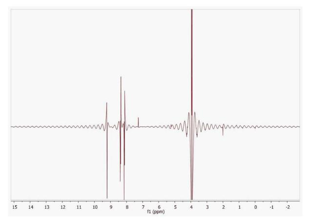
In order to work around this problem, Mnova reads the length of the group delay to be able to calculate the actual beginning of the FID to apply the required correction.
