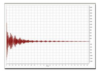
And this is the so-called **FID'**. In this case, prior to FT, Mnova applies a zero filling operation as can be appreciated in the FID' below. A zero fill increases the digital resolution by adding null data to the FID, increasing the size of the data array.
