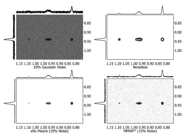
Comparison of the MMWF\* and eNL-means filter with a synthetic 2D spectrum 10% Gaussian noise (top-left). Top-right spectrum is the original noiseless spectrum whilst the two spectra at the bottom of the figure are the denoised spectra using MMWF\* (bottom-right) and eNL-Means (bottom-left)
