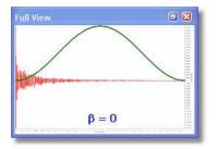
**First Point Correction:** There is an important difference between the *discreet* FT and the *continuous* FT. The *discreet* FT generates a constant vertical displacement of the baseline, which can be due to a
