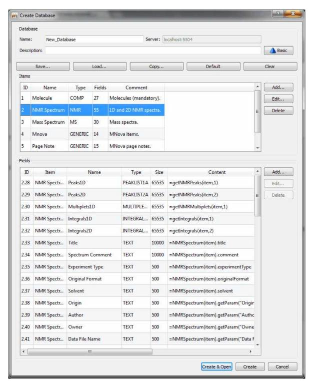
From here, it will be possible to define several fields for each object just by using small scripts (after having clicked on the 'Add...' button of the Field menu). For example in the example above, you can see how we have defined 40 fields for the object 'Spectrum', such as 'Peaks1D', 'Peaks2d', 'Multiplets1D, 'Title', etc. You can also get the information of the Database (showed in the picture above) just by following the menu 'Database/Database Info'
