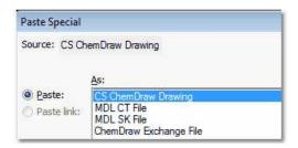
Indeed it will be possible to keep the numbering from ChemDraw or the abbreviated structures by using the 'ChemDraw Exchage file' from the dialog box above.
