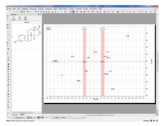
It is also possible to carry out assignments to 2D spectra by typing the applicable number of the atom in the 'Assignments Table' or **graphically** by selecting the atom in the molecule structure and the applicable signal in the 2D:
