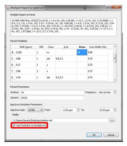
In the example above, we have assigned the multiplet at 5.29 ppm to the H-14 (and also the multiplets belonging to H-20' and H-20"), we loaded the mol file and checked the option to 'predict' the shape for those assigned multiplets. Here you can see the result:
