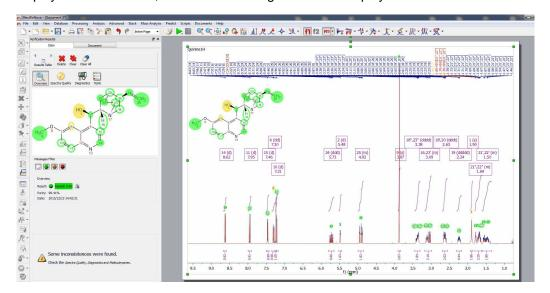
The paper area will present the spectra annotated with the assignments the software has made to the molecule and the molecule with each atom colour coded by quality of assignment (green is a good assignment, yellow is poorer assignment and red is a bad assignment but which still allows the software to make a total assignment of the structure).
