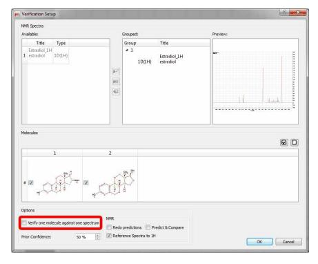
The software will run the spectral set against both structures and present the user with a score for each structural proposal, which may in many cases allow the user to differentiate between 2 possible candidate structures.
