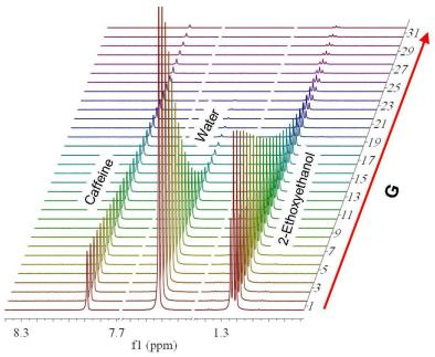
It can be observed that the intensities of the resonances follow an exponential decay. The slope of this decay is proportional to the diffusion coefficient according to equation (1). All signals corresponding to the same molecular species will decay at the same rate. For example, peaks applicable to water decay faster than the peaks of caffeine and 2-Ethoxyethanol
