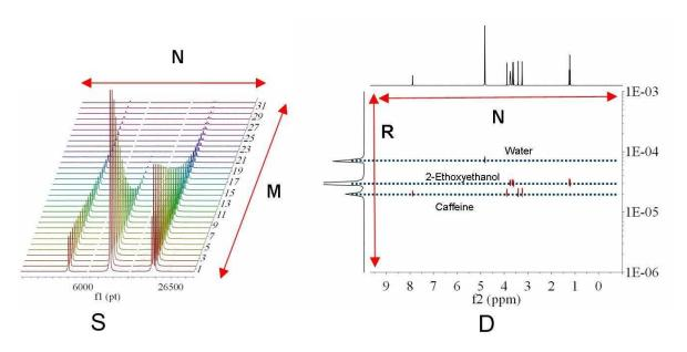
The horizontal axis of the DOSY map D is identical to that of S and encodes the chemical shift of the nucleus observed (general 1H). The vertical dimension, however, encodes the diffusion constant D. This is termed **Diffusion Ordered Spectroscopy** (DOSY) NMR. In the ideal case of non-overlapping component lines and no chemical exchange, the 2D peaks align themselves along horizontal lines,
