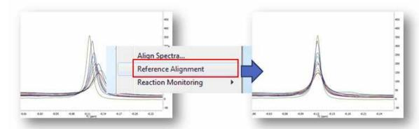
The idea of global alignment is very simple and corresponds to the well-known chemical shift referencing method in which the user sets the internal reference peak (e.g. TMS, DSS, TSP, etc) of each spectrum to e.g. 0 ppm. In order to cope with small fluctuations in chemical shifts, this method seeks for the highest peak within a narrow (user-defined, auto-tuning option in Mnova) interval, as depicted in the figure above.
