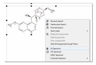
After that, you will obtain the desired predicted spectrum using a rigorous full quantum mechanics method taking into account any second order effect present in the predicted spin(s) systems(s):
