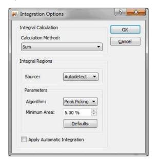
• Calculation Method: you can select between 'Sum' (classical integration, faster than 'Peaks' but without deconvolution), 'Edited Sum' or 'Peaks' (it takes into account only the integrals of the GSD spectrum and because of the deconvolution applied, it is slower than the 'Sum' algorithm). In the Peaks calculation method, it will be possible to select what peaks you want to take into account for the integration (for example, only compounds peaks and not solvent or impurity peaks, etc...)
