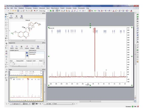
If your document has more than one molecule (<u>see also this tutorial</u>), it will be possible to select a different colour for the assignments of each compound by using the 'Compounds Table'. In the example below the assignments labels of the quinine appears in blue and the assignments labels of the EtOAc are green (make sure that 'Use Compound color' is checked in the Assignment Properties):
