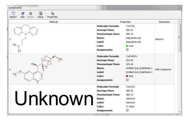
The user can type the name, label (to be displayed in the assignments) and molecular formula when creating a new unknown compound from the Compounds Table:
