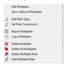
From here you will be able to display the 'Multiplet Manager' or the 'Table of Multiplets'. You can also change the 'Peaks Type' (from compound to impurity, solvent, artifact, etc) or to assign the peaks inside the multiplet to a specific compound. It will be also possible to generate a 'multiplet report', copy the multiplets to the clipboard, delete and add multiplet peaks, etc as you can see in the picture above.
