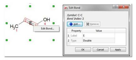
You can **change the atom** just by hovering the mouse over the atom and typing the applicable letter (i. e 'o' for Oxygen, 'n' for Nitrogen, "b" for Boron, 'b' plus 'r' for Bromine, or more complex labels, such as Me, Ph, COOH, etc). you can also change the atom by double clicking on it to display the 'Edit Atom'
