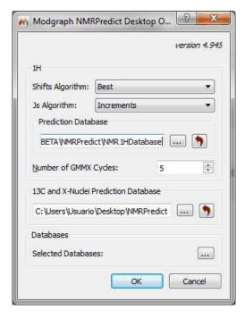
The 2D mol file representation of the structure is converted by <u>GMMX</u> into a 3D structure and then this structrure is repeatedly minimised to produce a series of conformers. The parameter "Number of GMMX Cycles" affect the number of conformers produced by GMMX. There is, however, no simple relationship between this value and the actual number of conformers.
