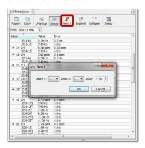
After that, the 'New J' dialog box will be displayed and you will only need to select the atoms involved in the coupling and the value of the new coupling constant. Click on OK and the new coupling constant will be added to the spectrum and also to the prediction table.
