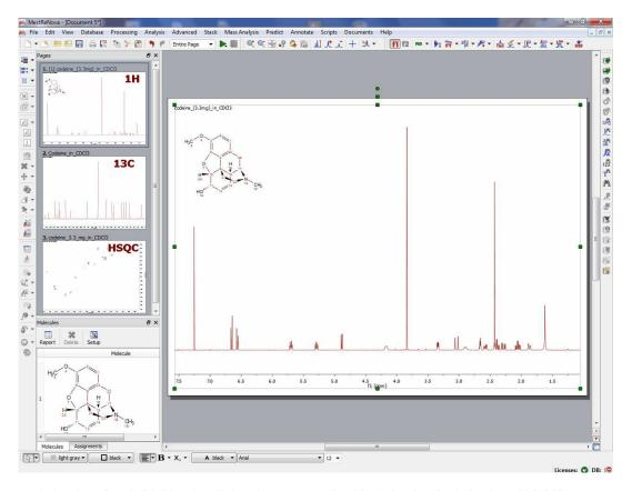
2nd: Apply a Peak Picking in all the datasets and a Multiplet Analysis in the 1H-NMR spectrum:
