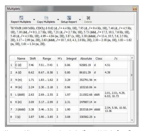
You can add/remove columns by selecting 'Setup table' in the Setup Report scroll down menu.
