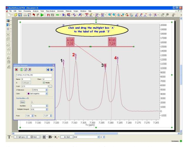
After that, the peak 3 will be a part of the multiplet A; (at this moment the multiplet A contains the peaks 1, 2 and 3):
