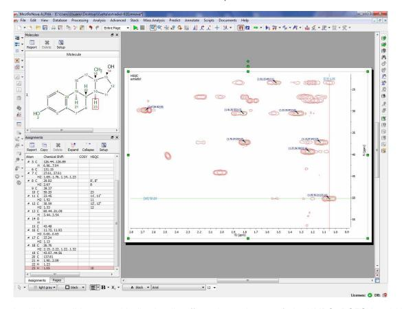
It will be possible to graphically visualize (from the assignments) the HMBC, ROESY and NOESY connectivity in the structure, by double arrows between the coupling groups. To do it, double click on the molecular structure to display the 'Properties' and select the 'Arrows' tab to check the desired correlation arrows:
