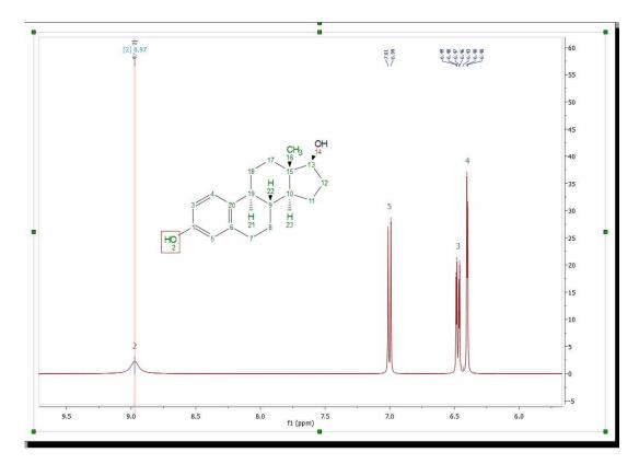
You will also notice that once the atom to peak assignment has been made, you will get an assignment peak label (over the applicable signal) with the number of the atom ([2] in the example above).
