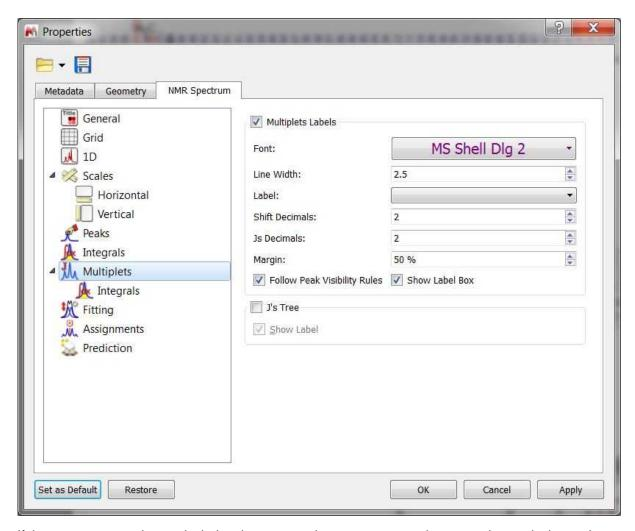
If the spectrum contains peaks belonging to more than one compound, we can show only the peaks assigned to one of them by <u>filtering</u> the desired peaks in the Peaks Table. Checking the 'Follow Peak Visibility rules' box will allow you to show only the multiplet boxes applicable to those visible peaks.
