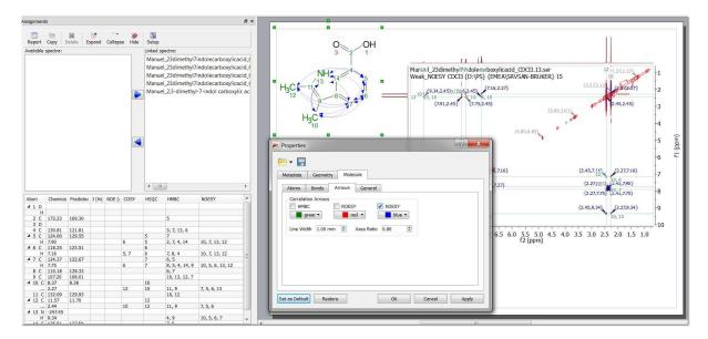
You can also copy several datasets in the same page (and after having resized them) to make the assignments. Here you can see a page which contains a 1H, 13C and HSQC datasets with an assignment in the molecular structure:
