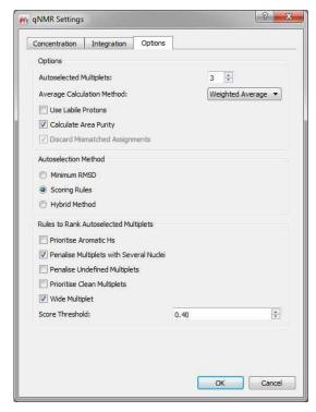
From here you will also be able to rank and prioritise multiplets as candidates for use in determining the concentration. They are based on empirical rules and penalties to give you the best chance of using a multiplet that is not "contaminated" with impurity peaks. (Labiles should almost always be excluded as they usually underintegrate).
