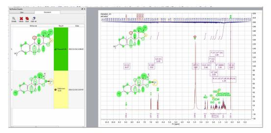
This is one of the areas where having the ability to combine NMR and MS data can prove very powerful. In the following example, 1H NMR alone does not distinguish between the structures on the total score, as the only difference is in a different nuclei (S or O) (although there are already some indications that one structural proposal has greater merit than the alternative in the quality of the assignments made by the verification module and reflected in the colour coding).
