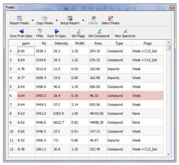
The Peaks table displays the list of peaks, including the following information: chemical shift in ppm and Hz, Intensity (height), Width (in Hz, at half maximum of the peak), Type (compound, solvent, impurity, etc), Flags, Multiplicity (for the carbons) and 'Annotations'.
