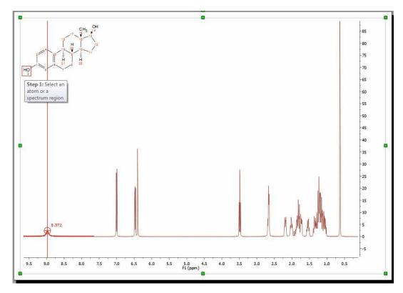
This peak will now be assigned to the atom (which will turn to green). Once the assignment has been made, you will get an atom number label on the chemical shift and hovering the mouse over the atom will highlight the applicable peak in the spectrum and hovering the mouse over the peak will highlight the corresponding atom on the molecular structure. To customize the assignments labels, click here.
