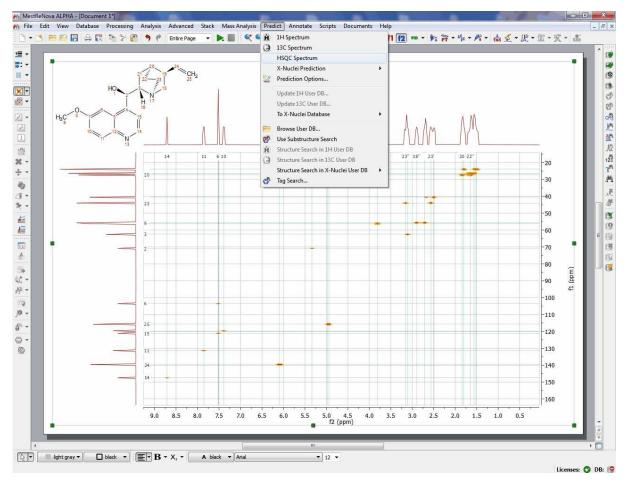
It is possible to modify the predicted chemical shifts either graphically, by clicking&dragging any prediction label, or by typing the new values in the prediction tables:
