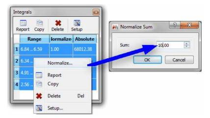
Double clicking on any cell of the 'range' or 'absolute' columns will display the 'Integral Manager', which will allow you to normalize or change the integral range:
