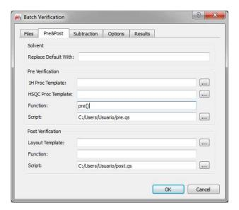
**Solvent/Replace Default With:** This allows users to handle situations in which the solvent may be wrong in the parameters. It can be the case that a certain batch has been run on a specific solvent but that the user left the default solvent on the spectrometer data entry and therefore the solvent could be wrongly entered. Since the target solvents will affect the performance of the Autoedit function in Mnova Verify, it is important to be able to correct for this at the script level.
