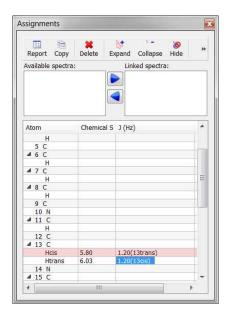
From the assignment table, it will be possible to delete any assignment by clicking on the Delete button after having selected the applicable cell in the table. To delete 'All the assignments' from the table, just do 'Ctrl+A' to select all the assignments and click on the Delete button. The same effect will happen if you follow the menu Analysis/Assignments/Delete All Assignments or if you right click on the molecule to display the context menu:
