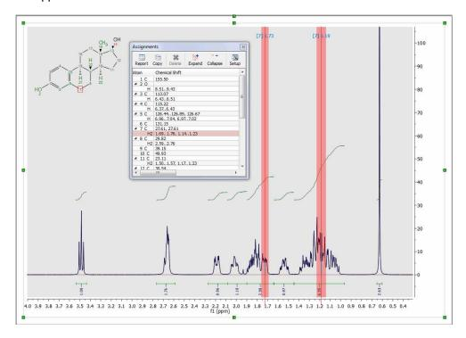
If you use the Assignment table to type directly the assignment of a CH<sub>2</sub> you would need add the prime marks if you want to assign only any of the two protons. If you do not type the prime marks, the assignment will be applied to both protons.
