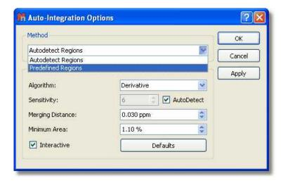
2. This will display a new dialog box, where the user will be able to select the desired ranges to apply the integration. If you have already integrated the spectrum you can click on the 'Use Current' button to import the integral ranges:
