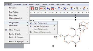
Mnova will automatically run a multiplet analysis and will fully assign your spectrum with the applicable molecular structure. If you have a license of the <u>prediction plugin</u>, the assignments will be more accurate.
