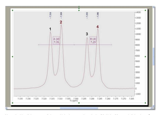
Next, double click on any of the multiplet boxes to launch the 'Multiplet Manager' dialog box. Once there, click on the 'Add multiplet peak' button (red square in the picture below). With this tool you can also remove peaks from the multiplet, by picking over a previously picked peak. It will also possible to delete undesired peaks by using this button .
