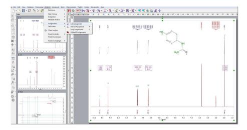
Mnova will automatically run a multiplet analysis and will fully assign your spectra with the applicable molecular structure. The multiplet boxes will be renamed with the corresponding atom number of the molecule and you will get an assignment label with the atom number over the applicable peak. In addition, hovering the mouse over the atom will highlight the applicable signal in the spectrum.
