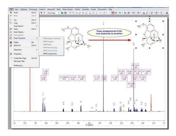
Another way would be to just copy&paste the molecular structure with the assignments and make the structural changes in one of the molecules. You could renumber the resulting molecules by selecting 'Concatenate Numbering' from the 'Molecular Drawing Toolbar':
