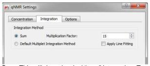
**Sum**: This will do a classical "sum" integration. To account to varying peak line-widths, we determine the line-widths and multiply this by the Multiplication Factor. This is used to always set sensible integral
