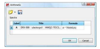
Where **A** corresponds to the real part of the original spectrum and **TRANS** indicates the transpose operation. This operation will produce the (unnormalized) Covariance NMR spectrum, in this case the 13C-13C correlation spectrum. Of course, in order to better approximate the covariance spectrum to
