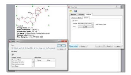
The molecule label is stored in a layout template and also gets applied when applying the template. See also the Properties chapter (for further information about the macro editor)
