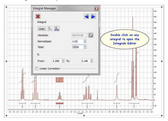
Currently it is possible to manually add integrals and multiplets using different integration calculation methods (Sum, Edited Sum and Peaks). To avoid missunderstandings in the integration results, it is possible to track the method used in each integral/multiplet. This will be displayed in the Integral/Multiplet Manager, where there is an option to recalculate each integral/multiplet with ability to choose the integration method in each case.
