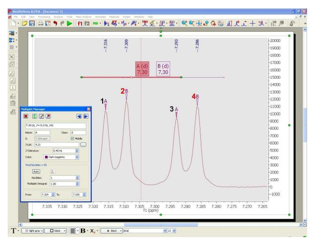
As you can see in the picture above the multiplet A contains the peaks 1 and 3 and the multiplet B contains the peaks 2 and 4.
