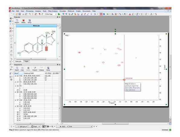
Once an assignment is made in a 2D spectrum, this assignment will be **transferred** to the applicable **multiplet** box in the 1H spectrum:
