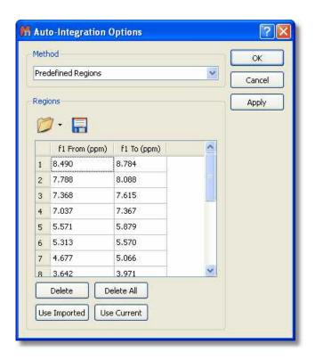
Clicking on OK, will apply the integrations to the current spectrum and keep the regions to apply further integrations to additional spectra by just clicking on 'Predefined Regions' in the Integral scroll down menu:
