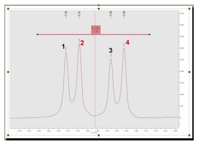
where the peaks 1 and 3 correspond to one doublet and the other peaks (2 and 4) to the second doublet. First of all, divide the multiplet just by clicking on the red square of the multiplet label (to obtain two overlapped multiplets):
