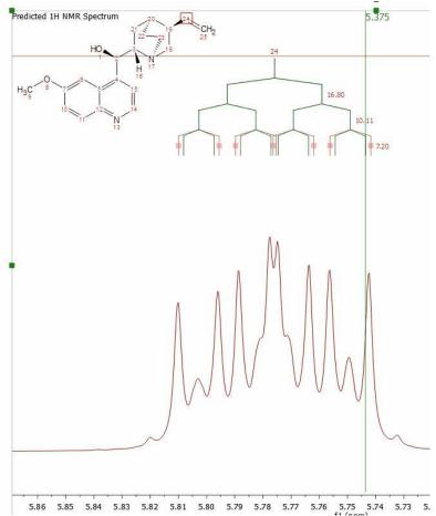
From the 1H prediction table is also possible to introduce new coupling constants. To do that just click on the on the 'New J' button
