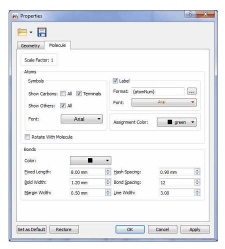
The 'Properties' dialog box will allow you to customize the size of the molecule, its angle with respect to the paper (geometry properties) and all representation properties, such as whether or not to show explicit carbon and hydrogen atoms, whether to show atom numbers, the length and spacing of bonds, etc. It is therefore possible to achieve many different representations of the same molecule, as the figure below shows.
