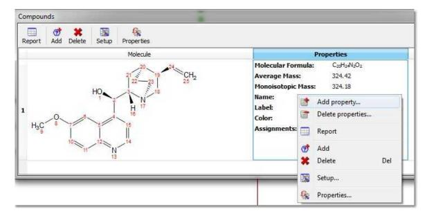
The added properties can be deleted in the same way, by selecting 'Delete Properties'. The visibility of these properties can be also customized via Properties button. By default the visibility is setup as automatic.
