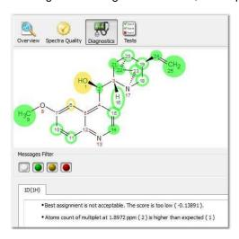
Clicking on the 'Tests button', will display the Score, Significance and Quality values for each individual test, which is designed to help you identify quickly possible reasons for a failure:
