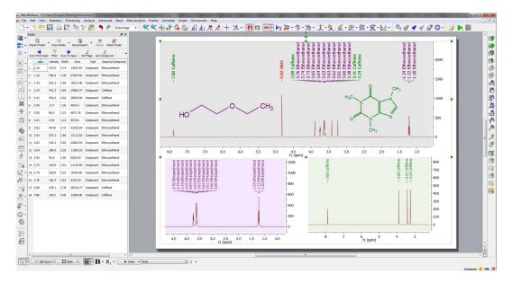
It is possible to edit automatically the Type and Flags of each signal, just by selecting 'Auto Classify Peaks' in the Peak Picking scroll down menu:
