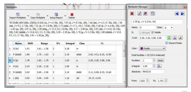
The user can paste the 'Multiplets' table on the spectrum by clicking on the 'Report table' option (under the 'Report Multiplets scroll down menu) and also can delete a multiplet from this table by using the 'Delete' icon when the undesired multiplet is highlighted.
