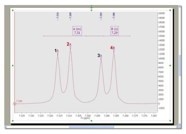
Finally, do the same procedure with the peak  $\bf 2$  and the multiplet box  $\bf B$  (click and drag the peak label to the multiplet box or vice versa), in order to include the peak  $\bf 2$  into the multiplet  $\bf B$ :
