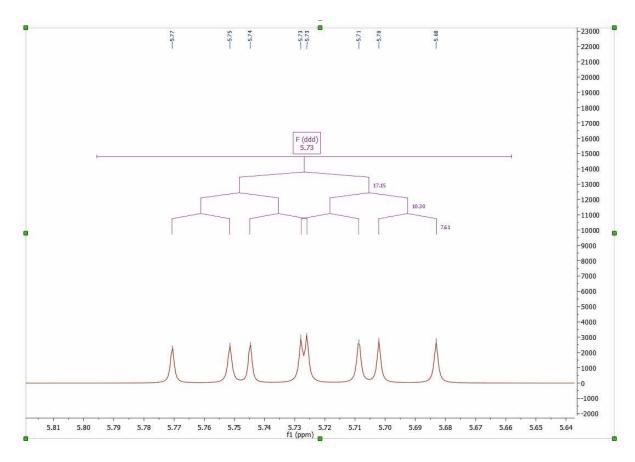
These objects are mouse sensitive in the case of predicted spectra, making possible the graphical edition of both the chemical shift and couplings by using drag & drop.
