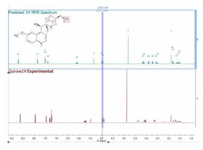
As you can see, you will get the predicted spectrum on top with the proton assignments labels. It could be possible to draw (or load) a second molecule over the 'Predict&Compare' result, in order to get a new prediction in the stack:
