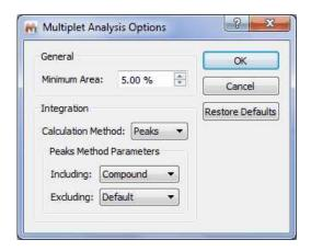
From here you can select the minimum area and the integration calculation method (Peaks, which uses GSD, or Sum, which is the classical integration method) and also to select what kind of peaks will be take into account for the multiplet analysis. By default **only compounds peaks** will be, so the solvent peaks will not affect to the multiplet analysis (very useful for example if a solvent signal overlaps with a compound peak).
