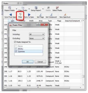
It will be also possible to synchronize the type of the peaks in the table (i.e: only Compounds peaks) with the peaks showed in the spectrum (by using the button 'Sync from Item') or viceversa, to synchronize the spectrum peaks with the peaks showed in the table ('Sync to Item' button).
