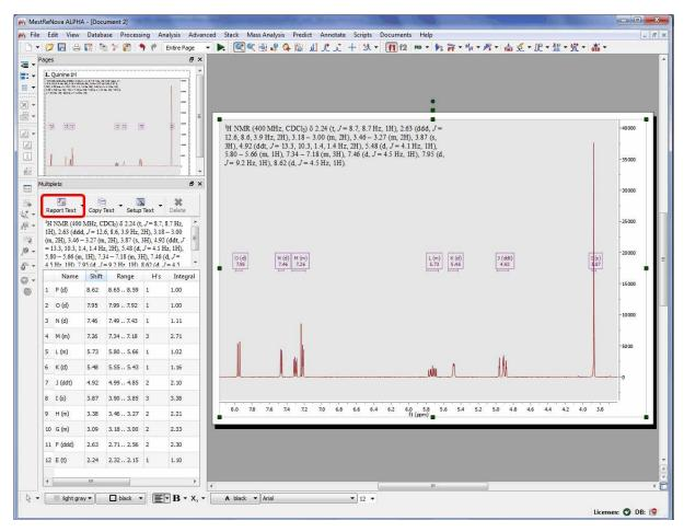
The same result will be obtained by right clicking on the multiplet box and selecting 'Report Multiplets' or by selecting 'Report Multiplets' in the 'Multiplet Analysis' scroll down menu (highlighted in red in the picture below). Of course, the user will be able to add an icon for this feature (highlighted in green in the picture below) into the toolbar. See the chapter 'Toolbars Customization' for further information about it.
