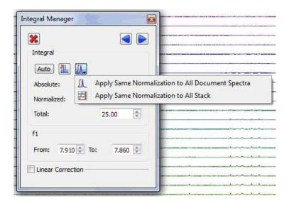
**Linear Correction:** Linear correction is basically a straight line built connecting the left and right boundaries of every integral in such a way that the final area will include only the integral above that line. In other words, if A is the total area under the peak(s) and B is the area under that straight line, the reported integral R will be:
