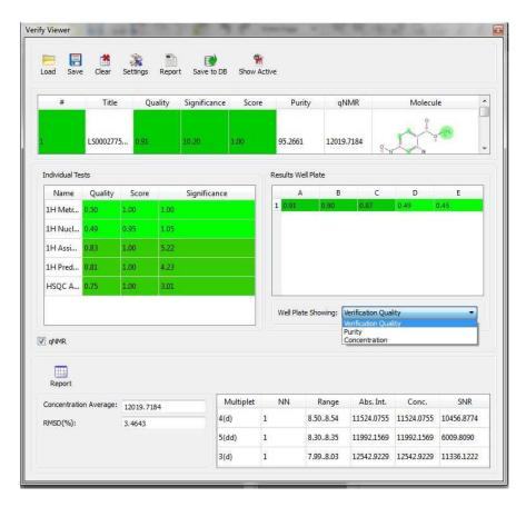
Clicking on the 'Settings' button will allow you to customize the fields that appears in the table, to save automatically the results to the Database and to create single Mnova and PDF documents with or without extended results:
