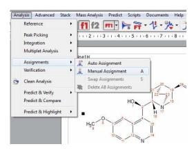
Finally, click on an atom in the molecular structure (or a spectrum region) and then release the mouse and drag it to your desired peak. Once your desired peak is highlighted on the spectrum, click on it to assign it.
