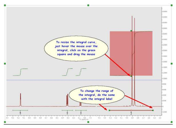
**Cutting Integrals:** It is possible to divide any integral just by clicking on the red square of the integral label and dragging the mouse as you can see in the picture below:
