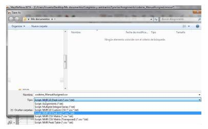
It is possible to export NMR spectra via 'File/Save As/NMR Custom CSV File' with options to export PPM+Re+Im, Hz+Re, PPM+Re or Hz+Re+Im, either from right to left or from left to right.
