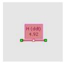
**Cutting Multiplets:** It is possible to divide any multiplet just by clicking on the red square of the multiplet label and dragging the mouse as you can see in the picture below:
