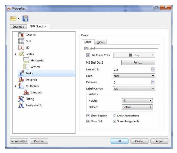
Then, the user can display or hide the peaks (according the peak type by selecting the applicable option in the scroll down menus) and to show/hide the Position, Annotations, Ticks or Assignments by checking (or unchecking) the applicable check box. It will be also possible to select the color, the font and the units (ppm or Hz) of the 'peak picking label'; the number of decimal figures to be shown on screen and the position of the 'peak labels'.
