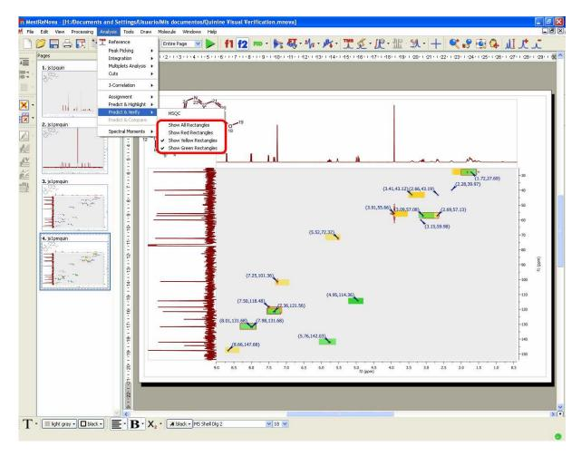
Bear in mind that the results reported by visual verification will depend on the prediction algorithm used in the spectral simulation. The user will be able to change this algorithm by following the menu: 'Predict/Prediction Options/Predictor Properties'.
