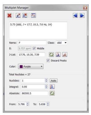
Currently it is possible to manually add multiplets using different integration calculation methods (Sum, Edited Sum and Peaks). To avoid missunderstandings in the integration results, it is possible to track the method used in each multiplet. This will be displayed in the Multiplet Manager, where there is an option to recalculate each integral/multiplet with ability to choose the integration method in each case.
