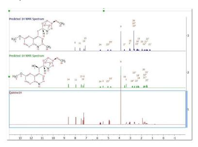
Hovering the mouse over the assignment labels and clicking&dragging will change the chemical shift in in real time:
