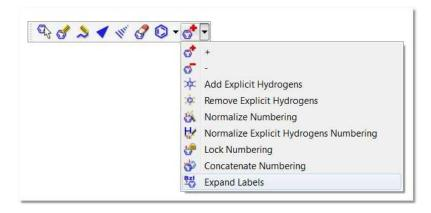
The **Normalize Numbering** button applies re-numbering of the whole selected molecule. From the <u>Preferences</u> you can select if you want to auto-renumber the imported (or pasted) mol files (and also when joining fragments); very useful if you have two equal molecules drawn in different applications or in different order, and you want to normalize the numbering.
