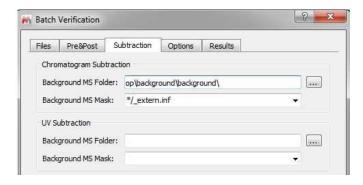
It will be possible to subtract chromatograms by scripting. This will allow users to subtract a blank background run from the run of interest, for example to ensure a good baseline for quantitation purposes, or to accurately measure differences between two or more runs.
