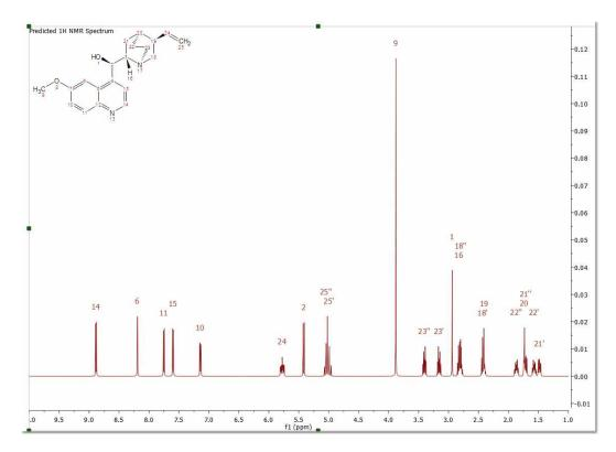
This predicted spectrum can be analyzed as a real one (e.g. it can be integrated, etc). The user can also visualize and edit the chemical shift and coupling constants values from the tables of the predicted spectrum by following the menu 'View/Table/1H Prediction'. Please bear in mind that the peak labels and the multiplet boxes will show the applicable atom numbers of the prediction.
