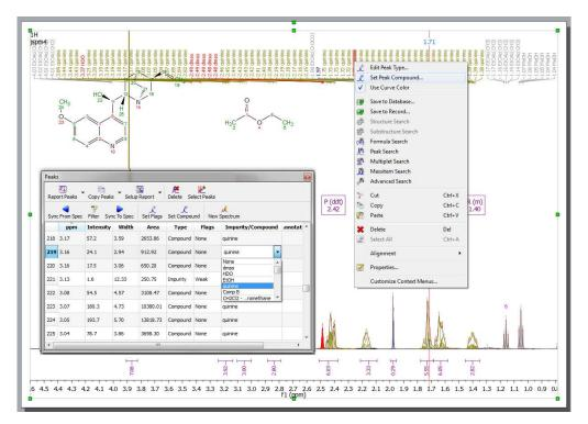
From the Peaks table it will be possible to apply some filter (by clicking on the applicable button) to show for example only Compounds Peaks. If the spectrum contains peaks belonging to more than one compound, we can show only the peaks assigned to one of them (by using the 'Filter' button):
