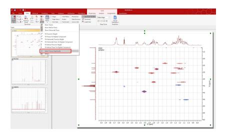
The user will be able to **'Fit Traces to Height'** (the vertical, the horizontal or both), just by following the menu 'View/2D Traces' or by using the **'Show Traces'** scroll bar menu on the left vertical toolbar:
