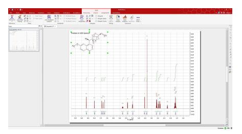
You can also modify the chemical shift and the coupling constant values from the table of the predicted spectrum. Just, highlighted the spectrum, follow the menu 'Prediction/1HPrediction Table' and then
