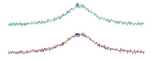
Parabolic interpolation and/or measurement of the intensity as the maximum height within a fixed box around the peak will help to minimize the effects of movements on the chemical shift position of the peaks due to, for example, temperature instability, pH changes, etc.
