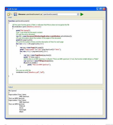
The object 'Application' of the variable **var** dW = new **DocumentWindow**(**Application.mainWindow**.activeWindow()); gives us the 'Active Window' of the 'Main Window', that is to say, the document which we can see in the screen. The function **print**(dW.pageCount()); is used to know the number of the pages of the document.
