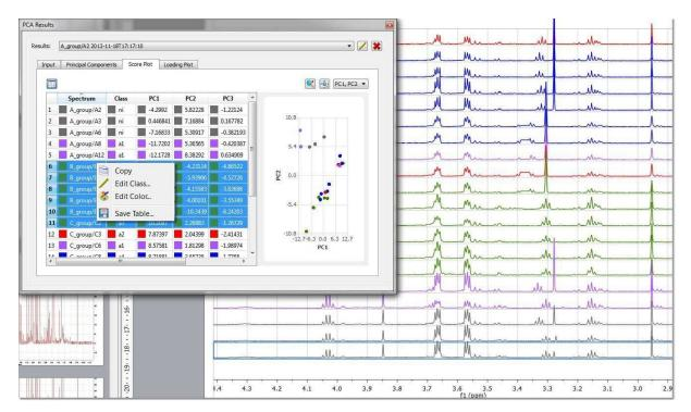
Select the applicable tab to display the 'Loading Plot'. In this plot, each point will be associated to each region of the stacked spectra. You can change the visibility and colors of the bins by right clicking on the applicable row:
