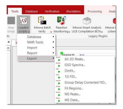
The script called 'All 2D Peaks' will export all the peaks of 2D datasets in the current document. The 'DmFit' will export 1D-NMR spectra to Dmfit ASCII format. The 'FID' script can be used to extract a XY text file for the FID. This script saves original FID independently on what is shown on the screen (FID, or FID', or FT Spectrum). The 'Fit Regions' script will export the fit peaks to a text file. The 'GSD Spectra' script will generate an ASCII file with the GSD peaks.
