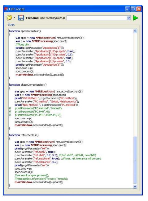
**Magnitude Active Spectrum script**: Let's see another script; in this case this script is used to obtain the 1D-NMR spectra in magnitude. Just open a 1D-NMR spectrum in Mnova, load this script by following the menu 'Script/Edit Script', type "magnitudeActiveSpectrum()" in the edit box and click on the green triangle to run the Script. You will obtain automatically your 1D-NMR spectrum in magnitude.
