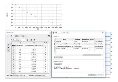
Follow the menu 'Analysis/Data Analysis/Edit/Fit to Best' and Mnova will try to guess the order of the reaction; fitting the data to standard equations and comparing the mean square error:
