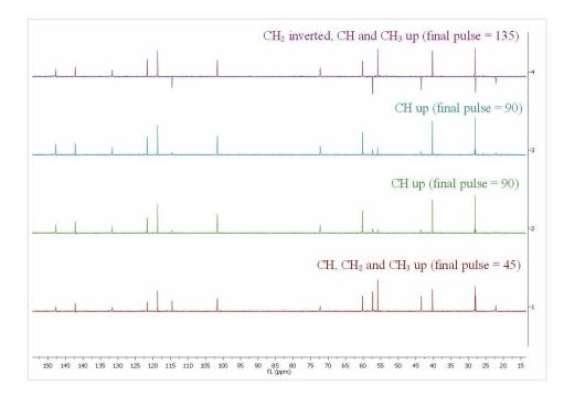
As you can see, you will have in the first slice (red slice with final pulse: 45 degrees) all the protonated signals, in the second and third slices you will get only the CH signals up and in the forth slice (purple slice with final pulse of 135 degrees) a spectrum with the CH and  $CH_3$  up and the  $CH_2$  down
