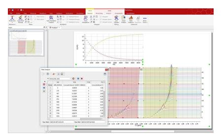
We can use the green square handlers to adjust the regions of interest with the deviation of the signals in the stacked (you could also use the <u>'Align Spectra'</u> feature)
