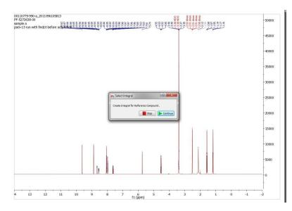
In that case, we will manually integrate the signal at 5.74ppm and click on the 'Continue' button:
