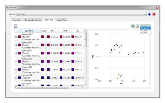
Each point of the 'Score Plot' is associated to a trace of the stack. If you are in the 'Active Spectrum' mode, you will get displayed the applicable spectrum when clicking on the point (of the Score Plot):
