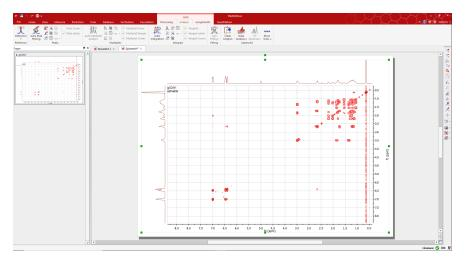
As you can see, this spectrum is not referenced. To apply an automatic referencing, just right click on one of the traces and select 'Setup' to display the 'Setup Traces' dialog box. Once there, select the desired external trace and check the applicable box (highlighted in red in the picture below):
