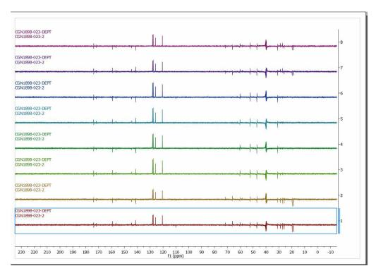
The arrayed variable mult '0.5 1 1 1.5' refers to the type of DEPT spectrum, in this case DEPTQ 45°, DEPTQ 90°, DEPTQ 90° and DEPTQ 135°, respectively
