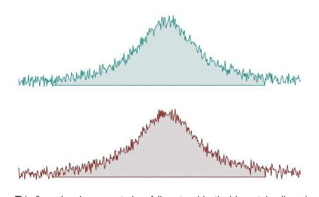
This figure has been created as follow: two identical Lorentzian lines (green & red) were simulated and then noise was added. The noise level is the same in both spectra but obviously, the actual numbers are different (more technically, noise in both spectra was calculated using a different seed in the random number generator).
