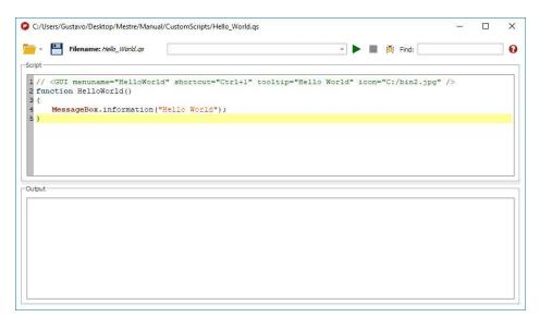
In this example we have defined a function called **helloWorld()** which will simply display a message box with the text 'Hello World'. Note that **MessageBox** is in bold, meaning that Mnova script editor recognizes it as a valid function.
