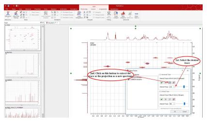
You can extract the vertical trace in a 2D spectrum and apply a FT on it. To get it:
