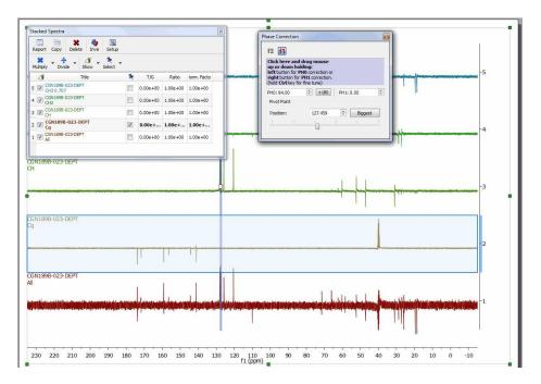
After having corrected the Phase to all the traces, this will be the result (from up to down: CH3, CH2, CH, quaternary and All carbons):
