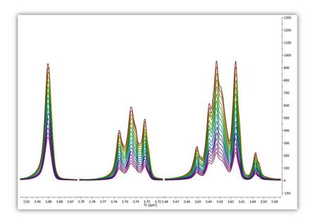
Finally, there is an additional display mode, the so called whitewashed stacked plot. The whitewashing effect means that the spectra at the front of the display hide the spectra behind them from view, as depicted in the figure below.
