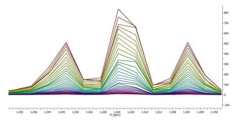
As seen in the figure above, binning clearly removes the effect of chemical shift changes but of course, at the cost of a significant reduction in data resolution.
