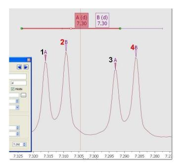
As you can see in the picture above the multiplet A contains the peaks 1 and 3 and the multiplet B contains the peaks 2 and 4.
