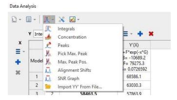
Please note that you can also change those options by double clicking on the '...' button of the Model cell under the Y(X) header of the Data Analysis panel:
