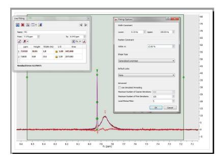
**Position Constraint:** it takes into account the values outside the range (p=shift) p\*(1-pos\_constraint\*p). A big value of the algorithm will 'shift' the peak far. Normally, you will not need to change the default value, because the peak should be close to the original position.
