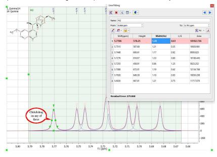
Clicking and dragging on the next two squares will modify the Lorentzian/Gaussian ratio of the signal and finally the last square will be used to modify the chemical shift of the signal.
