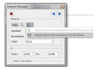
This is very useful if you need for example to determine relaxation times from a series of 1D spectra, to be able to compare the integral values between the different traces.
