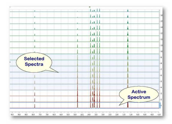
You can also **select** several slides by using the check boxes on the right of the 'Stacked Items Table'. When the spectra are selected, they are highlighted with a light blue background. Any processing operation will take place only for those selected spectra.
