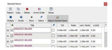
T/G column: 'T' stands for Time whereas 'G' stands for Gradient. The underlying idea is that the Data Analysis module is intended mostly to analyse (1) Reaction monitoring and relaxation experiments in which case the independent variable would be expressed in seconds and (2) Pulse field gradient (aca DOSY) experiments where the independent variable would correspond to field gradients strength.
