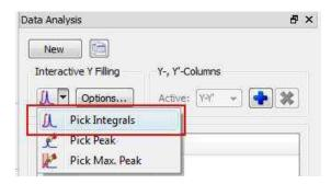
This method consists of a standard numeric integration over the whole peak. Basically, the program is summing up all the points within the selected area of interest) as illustrated in the figure below:
