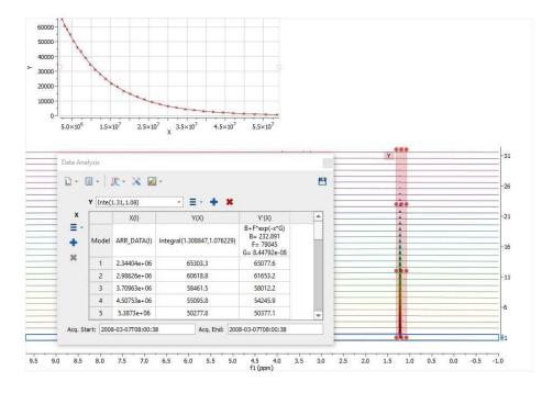
Please notice, that the integrated region will be highlighted in green and will contain several handlers to modify the ranges of the integration just by clicking&dragging them (which will be really useful for 'reaction monitoring' in order to account for peaks movements). Holding down the 'shift' key, whilst you click and drag on any of the handlers, will shift all the handlers together of the same vertical.
