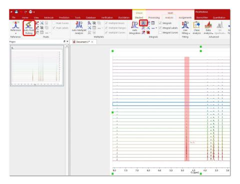
Then, just select 'Active Spectrum' under the 'Mode' scroll down menu to obtain only the highlighted spectrum and you will be able to see the integrals and the peak picking. To navigate through the traces, press and hold down **SHIFT** and use the up or down arrow keys (or the mouse scroll wheel):
