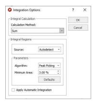
• Calculation Method: you can select between 'Sum' (classical integration, faster than 'Peaks' but without deconvolution), 'Edited Sum' or 'Peaks' (it takes into account only the integrals of the GSD spectrum and because of the deconvolution applied, it is slower than the 'Sum' algorithm). In the Peaks calculation method, you can select what peaks will be taken into account for the integration (for example, only compounds peaks and not solvent or impurity peaks, etc...)
