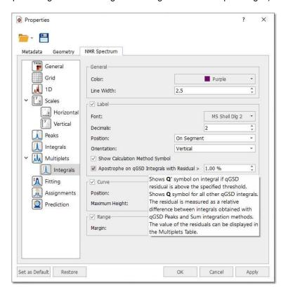
From here, you can also display the integral calculation method and also to label those integrals with a residual bigger than a value.
