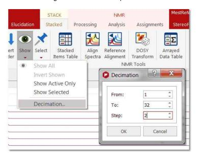
This option is very useful when the number of stacked spectra is very large, slowing down the plotting and not showing relevant information
