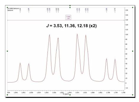
As it can be noticed, Mnova now finds an extra coupling of 11.4 Hz. If we take a closer look at the fine structure of the multiplet once GSD has been applied, we can observe that the 4 peaks in the center of the multiplet are actually split into 8 peaks as illustrated in the figure below:
