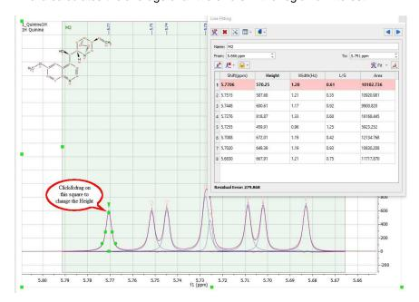
Clicking and dragging the green square at the top of the peak, will change the Height of the peak. The squares at the mid-height of the peak can be used to modify the Width of the peak:
