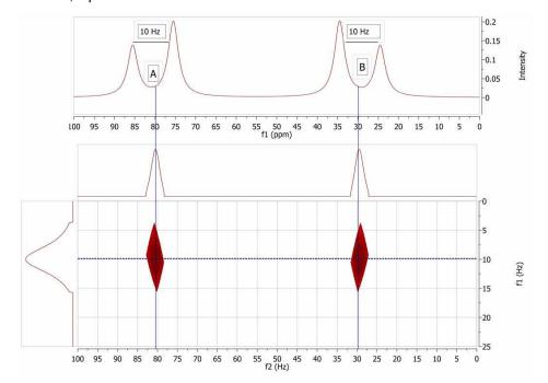
In this figure we have simulated 1D spectrum with two coupled spins, A = 80 Hz and B = 30 Hz. JAB = 10 Hz.
