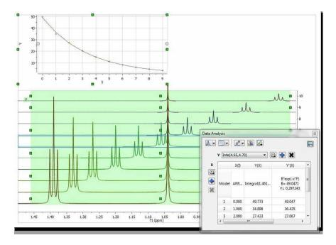
It can be noted that the graph shows an exponential decay, but the actual values must obviously be wrong as the values calculated, using the green rectangle as a boundary for the integration, include peaks from both the triplet and singlet, and we are interested in the analysis of the triplet resonances only.
