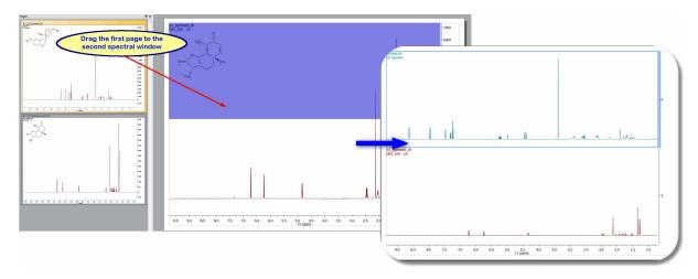
You can use this method to add a spectrum to an existing stack. In the example below we are adding the spectrum in the second page as the trace 19th of the stacked plot:
