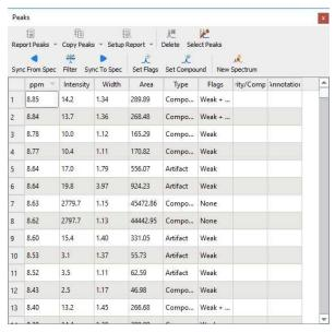
The Peaks table displays the list of peaks, including the following information: chemical shift in ppm and Hz, Intensity (height), Width (in Hz, at half maximum of the peak), Type (compound, solvent, impurity, etc), Flags, Multiplicity (for the carbons) and 'Annotations'.
