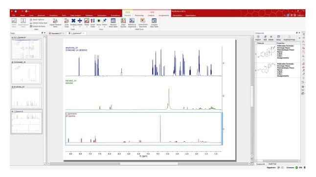
For metabolomics studies it is important to superimpose multiple spectra and compare their shape, e.g. to identify which ones are outliers. In such a mode, when the user sets a spectrum as the Active spectrum, that spectral curve will be displayed with a thicker curve. Follow the 'Home/Properties/Stack' menu to customize the 'Active pen width factor' (2.00 by default) and 'Secondary Transparency'.
