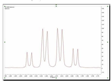
At first sight, this looks like a doublet quadruplet ( $J = 12.2 \times 3$ , 3.6 Hz) and in fact, this is what some NMR software packages would report if this multiplet were analyzed using based on traditional peak picking algorithms.
