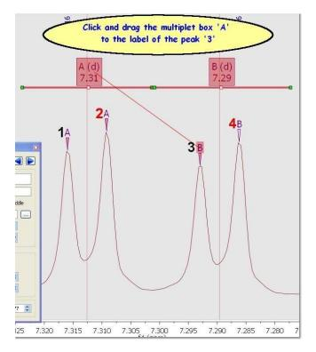
After that, the peak 3 will be a part of the multiplet A; (at this moment the multiplet A contains the peaks 1, 2 and 3):
