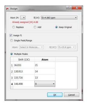
Alternatively, you could assign only one of the carbons and the next times that you need to assign carbons to the same proton, you will not need to select again the applicable proton (as it is already assigned). If you have overlapping in the proton dimension, you could hold down the Alt key and click to get the 'Assign' dialog displayed which will allow you to select any other proton.
