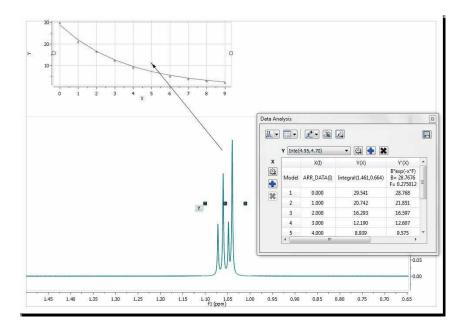
At this stage, there are several approaches. The simplest one is to just discard that point for the analysis, for example, by right clicking on that point in the graph and disabling it:
