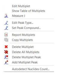
From here you will be able to display the 'Multiplet Manager' or the 'Table of Multiplets'. You can also change the 'Peaks Type' (from compound to impurity, solvent, artifact, etc) or to assign the peaks inside the multiplet to a specific compound. You can generate a 'multiplet report', copy the multiplets to the clipboard, delete and add multiplet peaks, etc as you can see in the picture above.
