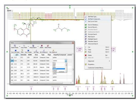
cell). The same effect will be obtained by right clicking on the Peak label and selecting 'Set Peak Compound' (please make sure that the 'Use Curve Color' box is checked in the 'Peaks Properties'):
