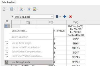
**IMPORTANT:** Every time a point is excluded, Mnova will *dynamically* recalculate the fitting function.
