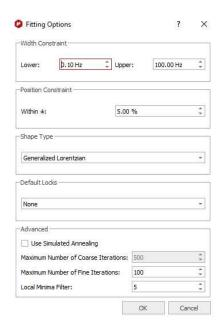
If the spectrum contains broad signals, just increase the Width Constraint to get good results. In the example below the Upper width constraint has been increased to 100 Hz:
