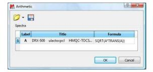
This arithmetic module is not restricted to matrix operations within a single spectrum. We can freely combine as many spectra as we want. For instance, if we have, in the one hand a COSY spectrum and in the other a HSQC spectrum, we can combine both in an analogous way so that the indirect covariance NMR spectrum yields a HSQC-COSY 2D spectrum.
