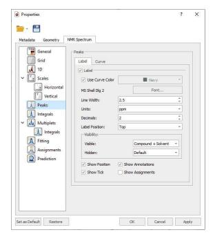
Then, the user can display or hide the peaks (according the peak type by selecting the applicable option in the scroll down menus) and to show/hide the Position, Annotations, Ticks or Assignments by checking (or unchecking) the applicable check box. You can select the color, the font and the units (ppm or Hz) of the
