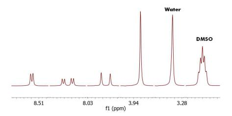
To remove the undesired peaks, just run a Peak Picking with GSD and with the 'Auto Classify Peaks' option enabled, in order to autodetect the solvent peaks (in yellow in the figure below):
