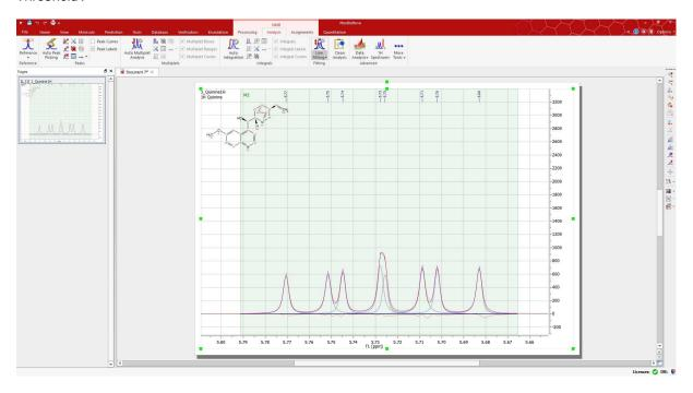
You can see in the picture above a blue line which corresponds with the fit peak, a red line which corresponds which the fitting residue and a magenta line which corresponds with the sum.
