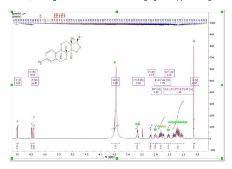
This algorithm for automatic assignment of NMR spectra has to be understood as a quick method to generate an initial 'rough' assignment that in some cases will require manual intervention from the user to easily amend any potential incorrect auto-assignment.
