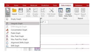
You will notice how the cursor will change to a blue integral. Now you will only need to integrate the desired signal (in this case, we will select the signal at 1.20 ppm). Once you have integrated the desired region, you will notice how the graphical will change according with the decay of the signal. Please bear in mind that all values will appear in a tabulated form in the <a href="Data Analysis panel">Data Analysis panel</a>
