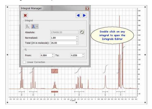
You can manually add integrals and multiplets using different integration calculation methods (Sum, Edited Sum and Peaks). To avoid missunderstandings in the integration results, you can track the method used in each integral/multiplet. This will be displayed in the Integral/Multiplet Manager, where there is an option to recalculate each integral/multiplet with ability to choose the integration method in each case.
