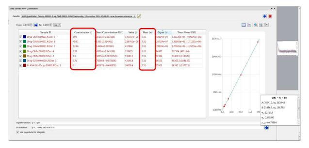
Automatically, we will get a calibration curve with a fit function which will be used to calculate the concentration of unknown samples. Statistic information can be displayed by clicking on the plus button besides the Fit Function.
