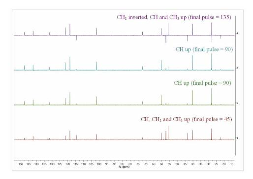
As you can see, you will have in the first slice (red slice with final pulse: 45 degrees) all the protonated signals, in the second and third slices you will get only the CH signals up and in the forth slice (purple slice with final pulse of 135 degrees) a spectrum with the CH and CH<sub>3</sub> up and the CH<sub>2</sub> down
