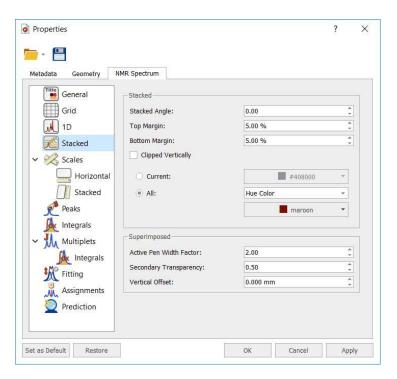
You can change the top and bottom margins of the stack plot, which is really useful in to avoid clipping a stacked plot at the spectrum border. With this property you will be able to adjust the distance between the top of the spectrum object and the baseline of the uppermost spectrum.
