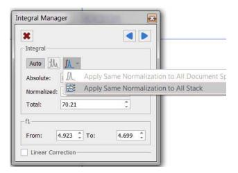
**Linear Correction:** Linear correction is basically a straight line built connecting the left and right boundaries of every integral in such a way that the final area will include only the integral above that line. In other words, if A is the total area under the peak(s) and B is the area under that straight line, the reported integral R will be:
