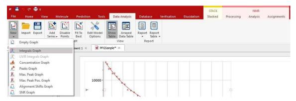
Its operation is very simple. The first thing you have to do is click on the New button. As a result, Mnova will populate the X-Y Table with some initial values (as described below) and create a new item, the so-called Data Analysis Plot. This new item will display the values from the X-Y Table which in general are the values extracted from the arrayed spectra, both experimental (Y) and fitted (Y').
