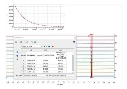
NOTE: the integration calculation method used in the Data Analysis will be the one selected under the 'Integral Options' (Analysis/Integration/Options).
