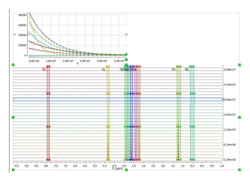
Follow the menu ' Data Analysis/Edit/Fit to Best' to allow Mnova to guess the order of the reaction (by fitting the data to standard equations and comparing the mean square error):
