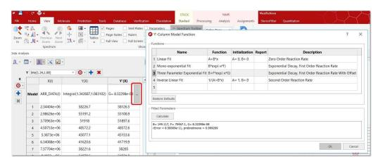
NOTE: The Probnotmono value is important to assess whether or not the model for the fit we are assuming, in this case, a three parameter-exponential model satisfies. For instance, if you assume a mono-exponential model but the experimental data follows a bi or multi-exponential behavior, then the analysis will not be fully correct.
