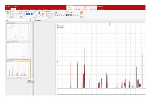
It is possible to apply any analysis feature (peak picking, integration or multiplet analysis) to the superimposed spectra and then take a look at the result over each trace by selecting 'Active Spectrum' in the 'Stacked' scroll down menu. To navigate through the traces, press and hold down **SHIFT** and use the up or down arrow key (or use the mouse scroll wheel)
