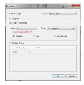
If you are working with a HMBC, you could assign one of the protons and then all the 13C in the same step (by selecting 'Multiple Peaks' from the panel):
