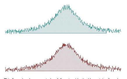
This figure has been created as follow: two identical Lorentzian lines (green & red) were simulated and then noise was added. The noise level is the same in both spectra but obviously, the actual numbers are different (more technically, noise in both spectra was calculated using a different seed in the random number generator).
