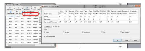
Purity (as a ratio of Compounds Vs (Impurity+Artifacts) peaks) can be displayed in Peaks table by selecting the checkbox "Show Purity Label" in Setup Table (disabled by default).
