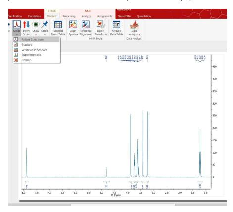
Finally you can export the peak picking or the integration analysis to a text file by following the menu File/Save as/Script:ASCII Matrix or 1D Integral Series (\*.txt). This will generate a text file which can be
