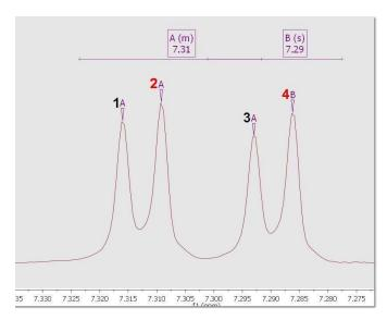
Finally, do the same procedure with the peak  $\bf 2$  and the multiplet box  $\bf B$  (click and drag the peak label to the multiplet box or vice versa), in order to include the peak  $\bf 2$  into the multiplet  $\bf B$ :
