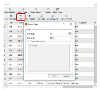
You can synchronize the type of the peaks in the table (i.e: only Compounds peaks) with the peaks showed in the spectrum (by using the button 'Sync from Item') or viceversa, synchronize the spectrum peaks with the peaks showed in the table ('Sync to Item' button).
