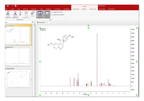
2nd: Apply a Peak Picking in all the datasets and a Multiplet Analysis in the 1H-NMR spectrum:
