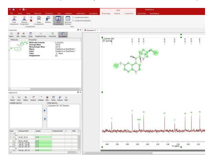
If your document has more than one molecule (<u>see also this tutorial</u>), use the compounds table to select a different colour for the assignments of each compound. In the example below the assignments labels of the quinine appears in blue and the assignments labels of the EtOAc are green (make sure that 'Use Compound color' is checked in the Assignment Properties):
