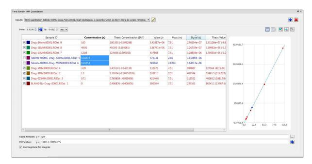
As you can see in the screenshot above, the known references used for the calibration curve appear in red and with the check box selected, whilst the samples to analyze appear in blue and unchecked.
