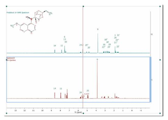
If you load a 1H-NMR spectrum with a multiplet analysis and run Predict and Compare; you will get a stack plot with the multiplet boxes displayed in the experimental spectrum, so you can easily assign those multiplets to the molecular structure and finally update the 'Prediction DB' if you wish:
