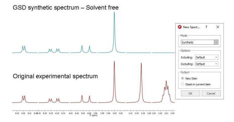
Here you can see another example where the solvent and compound signals are overlapped. Mnova's autoedit successfully separates a triplet signal sitting on the HDO signal. The approach of generating dark regions used by other software products would miss the triplet at 3.5 ppm and therefore any verification efforts would fail.
