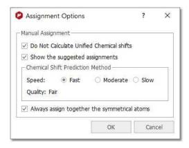
From the dialog above, you can also select the prediction algorithm used for the 'assisted assignment mode' and you will have an option to always assign together the symmetrical atoms.
