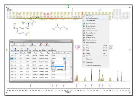
You can apply some filters to show for example only Compounds Peaks. If the spectrum contains peaks belonging to more than one compound, you can show only the peaks assigned to one of them (by using the 'Filter' button):
