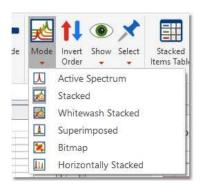
'Active Spectrum': to see only the highlighted spectrum. Within this mode, you can navigate along all spectra in this stack by using Shift+Mouse wheel (or arrow keys up&down).
