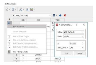
Copy the values from an an Excel worksheet and paste them into the X(I) column by highlight the first cell (in the row 1) and doing 'Ctrl/Cmd+V' to paste the values.
