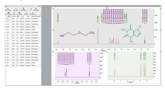
Select 'Auto Classify Peaks' in the Peak Picking scroll down menu to edit automatically the Type and Flags of each signal:
