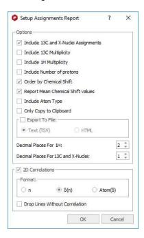
It is required at least a 1H spectrum. The table only will include columns for the spectra present in the document containing assignments. It generates a table in which each row corresponds to each non-equivalent proton.
