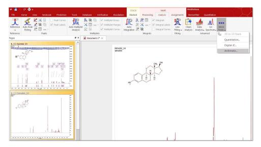
This will display the 'Arithmetic' dialog box on screen. In this example, we want to add two times spectrum A to spectrum B, so we shall type the formula 'A+2B' in the applicable cell.
