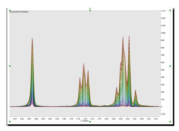
For metabolomics studies it is important to superimpose multiple spectra and compare their shape, e.g. to identify which ones are outliers. In such a mode, when the user sets a spectrum as the Active spectrum, that spectral curve will be displayed with a thicker curve:
