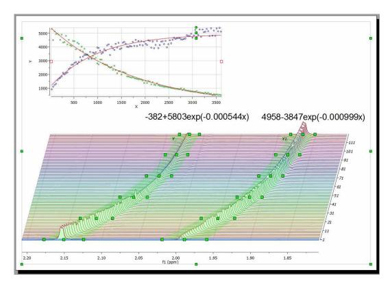
Clicking on the first cell of the column Y'(X) will allow you to fit the curve. In this case, we will fit it as a three parameter exponential curve.
