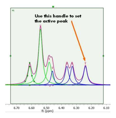
Any of these parameters can be locked for the Fit, just by double clicking on the applicable cell of the panel and closing the lock which appears. In the picture below it is shown how we have locked the width parameter of the peak 1 and also the L/G ratio of all the peaks, so these parameters will not change when the fitting will be applied. So a lock in front of a value indicates that it will not be optimized in the fitting.
