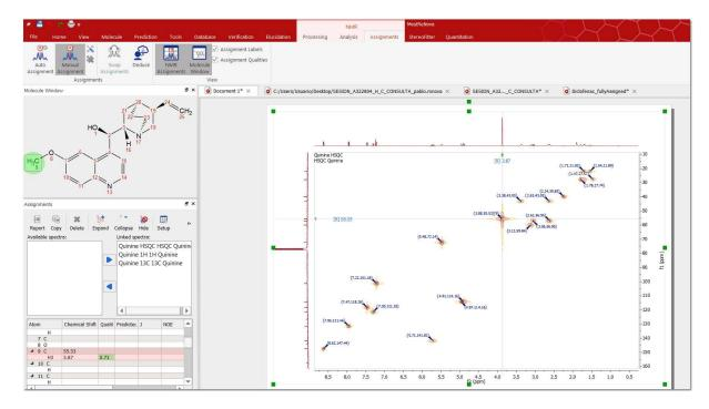
Once an assignment is made in a 2D spectrum, this assignment will be **transferred** to the applicable **multiplet** box in the 1H spectrum:
