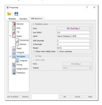
If the spectrum contains peaks belonging to more than one compound, we can show only the peaks assigned to one of them by <u>filtering</u> the desired peaks in the Peaks Table. Checking the 'Follow Peak Visibility rules' box will allow you to show only the multiplet boxes applicable to those visible peaks.
