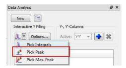
By default, the program will find the peak intensity at the position indicated by the user (using a vertical cursor) and then it will perform a parabolic interpolation in order to refine the value. In addition, the user can specify an interval in such a way that the program will find the maximum peak within that region. This can be done in 2 different ways:
