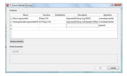
This dialog provides two predefined functions useful for fitting mono-exponential data (such as PFG and Relaxation NMR experiments) using either a 2- or a 3-parameter fit. Furthermore, this dialog offers the possibility to enter user customized functions.
