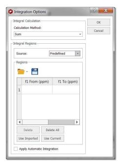
2. This will display a new dialog box, where the user will be able to select the desired ranges to apply the integration. If you have already integrated the spectrum you can click on the 'Use Current' button to import the integral ranges:
