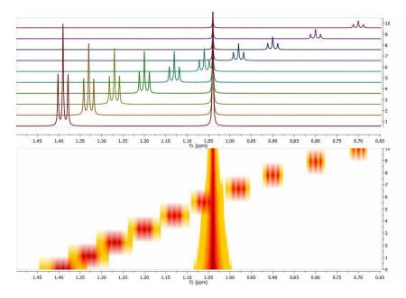
Now let's say you are interested in extracting the intensities of the triplet as the reaction progresses. There is actually no need to pre-align the spectra algorithmically; it is much simpler to have some kind of graphical tool to instruct the software which peaks (or multiplets) need to be used for the reaction monitoring analysis. Let me show you how this works in Mnova:
