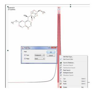
The user will be able to highlight in the table any desired peak just by clicking on the 'Select Peaks' button and then selecting the peaks in the spectrum (by clicking and dragging); then the user will be able to modified their flags (or Type) by clicking on the 'Set Flags' button. In the example below, we have changed the type of two peaks (from compound to impurity):
