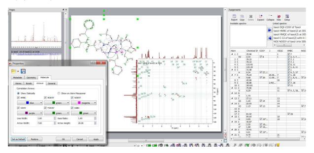
The Assignments table shows checkboxes for each row in the correlations that can be displayed as arrows in the molecule. Checking/unchecking these checkboxes will change the visibility of the correlations for each atom.
