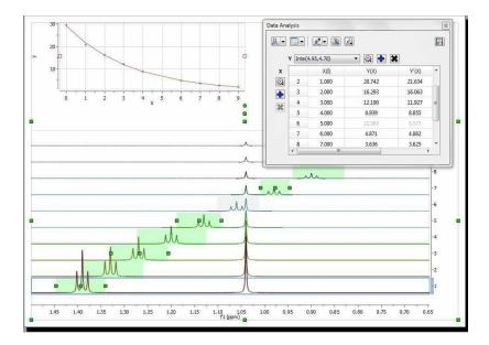
Another approach would involve using GSD to eliminate the singlet from the triplet so that it would not be necessary to discard the information from that particular spectrum.
