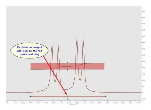
**Integration Manager (shortcut: Shift+I):** The integral editor will be displayed by double clicking on any integral curve, as you can see in the figure above. From there, you can change the integral range, normalize the integral to a specific integral, navigate through them and also to reference integrals to the total integral value for the spectrum.
