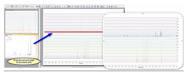
You can also create a stack plot by selecting the desired spectra in the page navigator (by holding down 'CTRL/Cmd key' while clicking on each spectrum) and then issue the command 'Stack/Stack Items':
