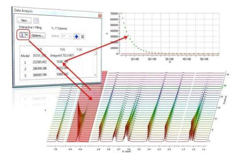
• Manual selection: if you take a closer look at the Data Analysis table in the figure above, you can appreciate that once the integral region has been selected, the program shows the following text: Integral(4.752, 4.907). This means that we have selected an integral covering that range. This value can be edited manually so that you can specify the limits by simply editing that cell.
