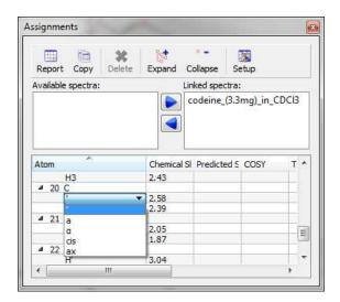
You can do **ambiguous assignments** in a -CH2, just by typing both values in the chemical shift cell (both chemical shifts are assigned to both protons)
