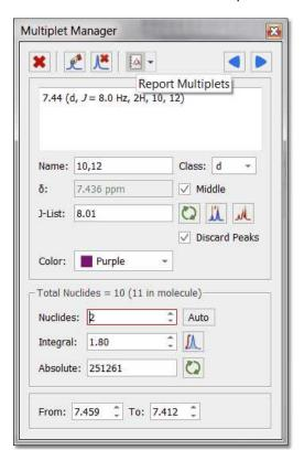
You can manually add multiplets using different integration calculation methods (Sum, Edited Sum and Peaks). To avoid misunderstandings in the integration results, you can track the method used in each multiplet. This will be displayed in the Multiplet Manager, where there is an option to recalculate each integral/multiplet with ability to choose the integration method in each case.
