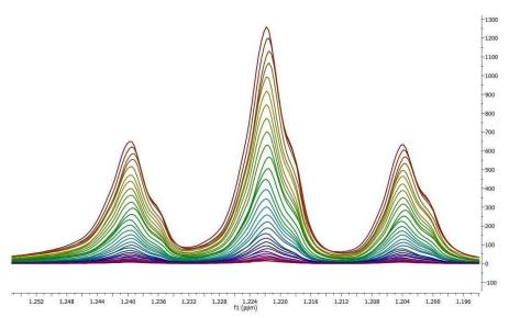
If peak heights are determined at a fixed position, this might introduce appreciable errors in the posteriori quantitative analysis (e.g. exponential fitting). As described before, this could be circumvented in some extent by using parabolic interpolation or peak searching of the maximum in a predefined box.
