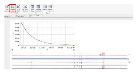
For convenience, you can **exclude points from the left and right** edges of the graph (by selecting 'Use Fitting Limits' on the Data analysis panel and highlighting the graph):
