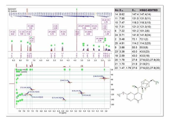
You can export the assignments as an ASCII file by following the menu 'File/Save As/Script:Assignments' or copy the assignments from one molecule to another (with the same numbering of the common parts).
