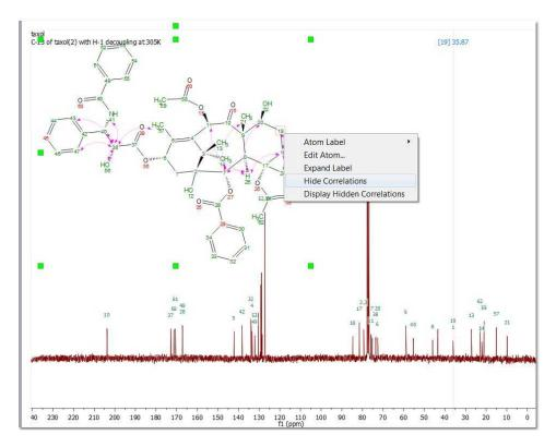
You can also copy several datasets in the same page (and after having resized them) to make the assignments. Here you can see a page which contains a 1H, 13C and HSQC datasets with an assignment in the molecular structure:
