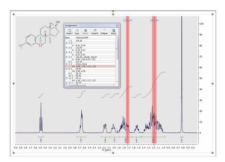
If you use the Assignment table to type directly the assignment of a CH<sub>2</sub> you would need add the prime marks if you want to assign only any of the two protons. If you do not type the prime marks, the assignment will be applied to both protons.
