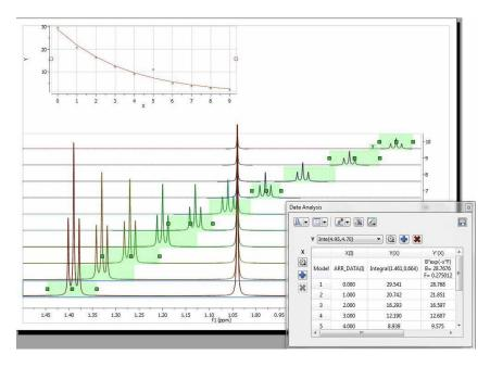
Now you can see that there is an outlier in the exponential curve which, obviously is caused by the singlet which overlaps with the triplet (spectrum number 6 which corresponds to data point #5, as in the graph the numbering starts from zero). Figure below shows that particular spectrum showing the singlet overlapping with the triplet:
