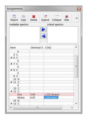
Click on the 'Delete' button to delete any assignment selected on the table. To delete 'All the assignments', do 'Ctrl/Cmd+A' to select all the assignments and click on the Delete button. The same effect will happen if you follow the menu 'Assignments/Delete All Assignments' or if you right click on the molecule to display the context menu:
